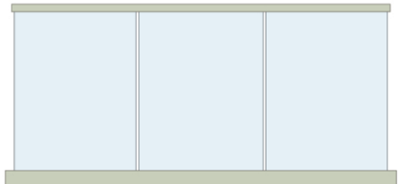
Glass balustrade with No Top Rail - must be approved by the local code official.
